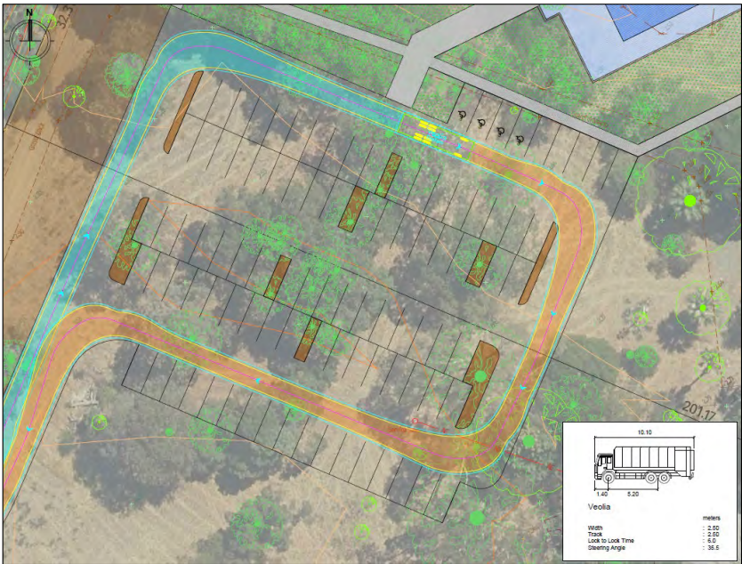
Figure 18 Swept Path Analysis – Waste Truck Internal Circulation
